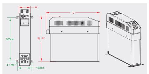
Note: mounting distance between two capacitors ≥ 50mm
