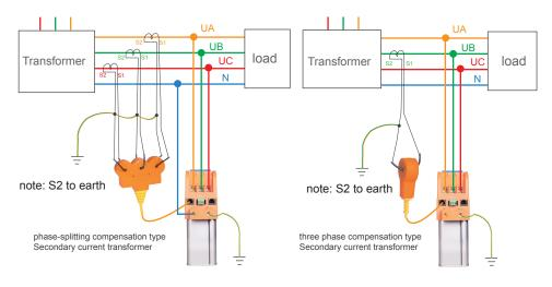
phase-splitting compensation type capacitor
